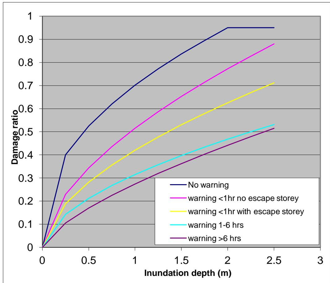
**Figure 5:** Content fragility curves for residential buildings for different warning lead times
