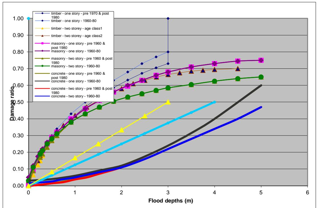
**Figure 1** Flood fragility curves for various building types, with inundation depth above the floor level (m) along the horizontal axis and average damage ratio along the vertical axis.
