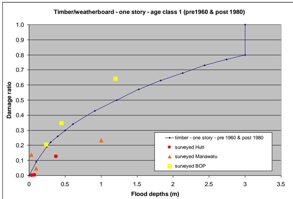
**Figure 3:** Comparison of fragility model and loss data for timber houses. Flood depth is relative to the floor level.
