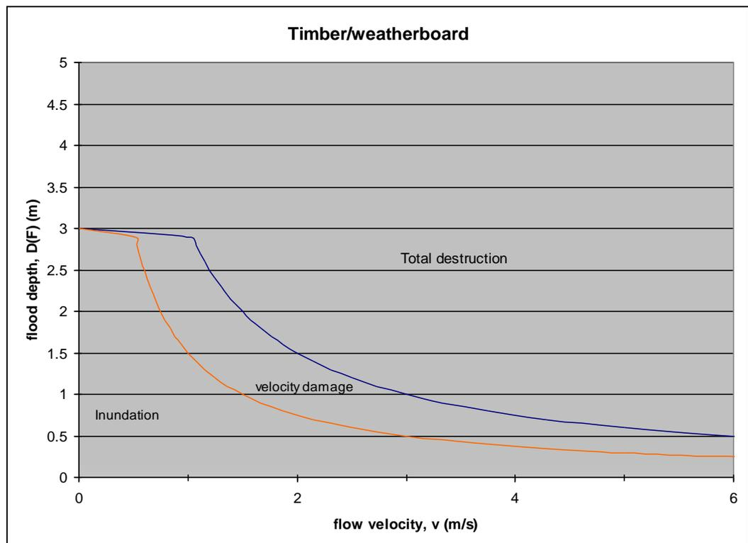
**Figure 2:** Inundation depth (D) and velocity (V) thresholds for: (a) onset of damage due to water velocity; and (b) total destruction, of timber / weatherboard buildings.
