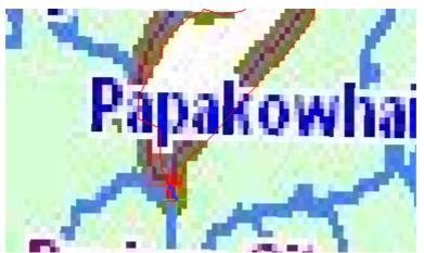
Five control points added. Zoomed in to better find the matching locations on the raster and vector layers. The differences between the red and green cross hairs is the error in the georeferencing. The image and the vector layers are unlikely to match exactly.
