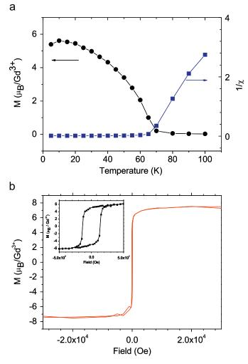
**Fig. 4.** Temperature-dependent magnetisation and inverse susceptibility in an applied field of 25 mT (a) and field-dependent of the magnetisation at a temperature of 10 K (b) of a 14 nm thick GdN layer. The inset is a magnification of the magnetisation at low field showing a coercive field of about 125 Oe.
