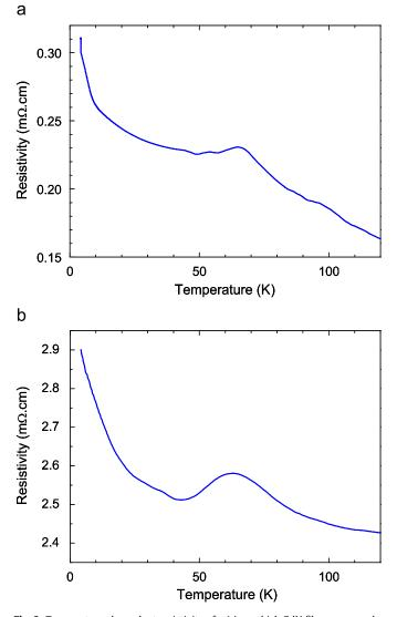
Fig. 6. Temperature-dependent resistivity of a 14 nm thick GdN film grown under (a)  $4\times 10^{-5}\, Torr$  of  $N_2$  and (b)  $4\times 10^{-4}\, Torr\, N_2$  with a peak at the Curie temperature.
