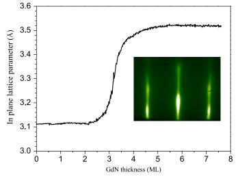
**Fig. 1.** Variation of in-plane surface lattice parameter during the growth of GdN on AlN as measured by RHEED. The inset shows the RHEED pattern along the Si [1 1 0] azimuth of a 14 nm thick GdN layer.
