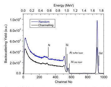
**Fig. 3.** Rutherford backscattering spectroscopy measurements in random (blue) and channelling (black) conditions of AlN/20.5 nm GdN/AlN/Si(1 1 1) sequence. The lines (labelled Gd, Al, Si and N) indicate the onset of backscattering energy for these elements at the surface. (For interpretation of the references to colour in this figure legend, the reader is referred to the web version of this article.)
