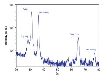
**Fig. 2.** X-ray diffraction scan of an AlN-capped 14 nm thick GdN film grown on an AlN/Si(1 1 1) sequence under  $4 \times 10^{-5}$  Torr of N<sub>2</sub>. This typical  $\Theta$ -2 $\Theta$ -scan XRD scan shows that in addition to the peaks of AlN and Si only the (1 1 1) and (2 2 2) reflections of GdN are present in these films. These data demonstrate the wurtzite (0 0 0 1) surface of the AlN buffer layer favours the growth of fully (1 1)-oriented GdN film.
