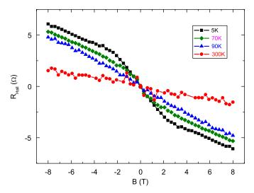
Fig. 5. Hall resistance for the 14 nm thick GdN films grown under  $4\times 10^{-5}$  Torr of  $N_2$  as a function of applied field at different temperatures 300, 90, 70 and 5 K showing the transition between paramagnetic and ferromagnetic phases.
