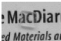
Photograph of one of the transparent polycrystalline fluoroperovskites.
